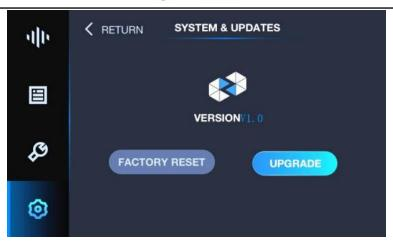
**Note:** Factory Reset only resets LAN and alias, but will not modify light calibration or firmware version, local files, and the work time of LCD/LED/PUMP.
