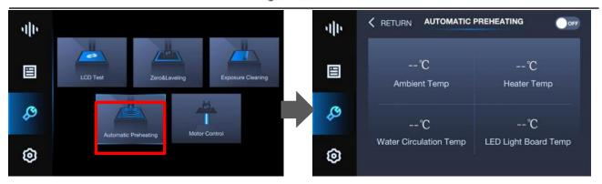
**Note:** only enable this when there is resin in the resin tank.
